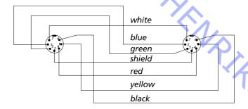
7-pin DIN cable for connection of audio and video systems:
