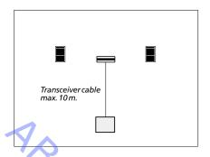
The cable between the transceiver and the relay box must not exceed 10 m. 5 m is mounted ex factory.
