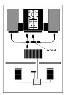
Beosystem 2300/2500 do not have a built-in output amplifier, and consequently a BeoLink System cannot be immediately connected to a Beosystem 2300/2500.
