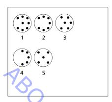
Used with Datalink and Power Link cables. **DIN plug, male**
