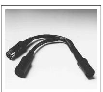
Used for connection between MCL 2P and Beosystem 2300/2500 and serial connection of active speakers.
