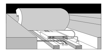
If it is not possible to place the relay box concealed in the attic or under the floor, it can be flush-mounted in the wall, using a flush-mount box.
