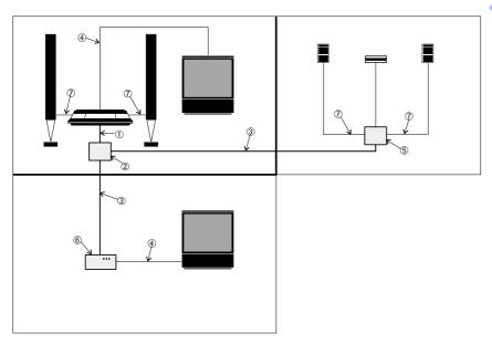
The illustration shows a visible installation, executed according to the star distribution principle.
