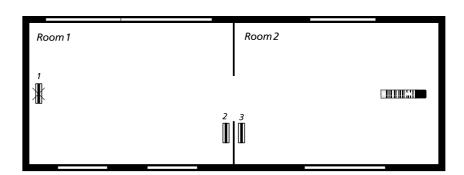
The diagram shows that transceiver 3 is placed appropriately, whereas transceiver 1 can be activated from room 2. Transceiver 1 should be placed as transceiver 2 instead.
