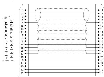
pin 1 = audio out, right channel pin 2 = audio in, right channel pin 3 = audio out, left channel pin 4 = audio ground pin 5 = blue groundpin 6 = audio in, left channel pin 7 = blue signalpin 8 = 12V sense and Datalink pin 9 = green ground pin10 = data 2pin11 = green signal pin12 = data 1pin13 = red groundpin14 = fast blanking, ground pin15 = red signalpin16 = fast blanking pin17 = video out, ground pin18 = video in, ground pin19 = video out, signal pin20 = video in, signal
