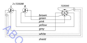
MCL cable between audio system and 8-pin wall socket:
