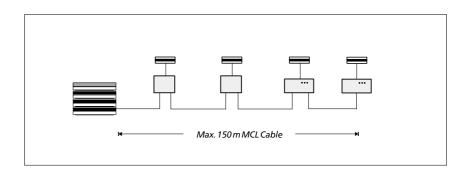
If the number of MCL 2 units is increased, or if more than 150 m of cable is used, it is necessary to insert an MCL 2 Expander.
