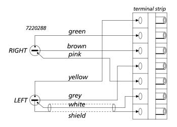
MCL cable between audio system and 7-pin terminal strip:
