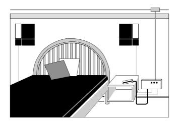
The socket panel may be placed inconspicuously, e.g. at the skirting of a wall
