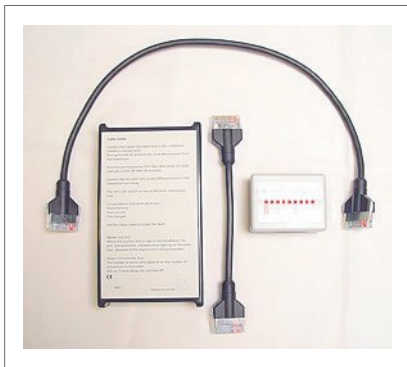
Professional tool for troubleshooting ML/PL installations. Circuit tester for connections/cables and sockets.
